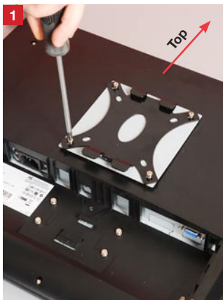
Attach the holder to the LCD...
