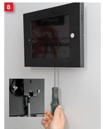
For extra security lock the LCD with the screw.
